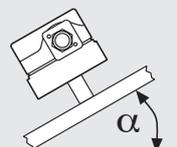
**When installed in an intermediate installation position, the pressure switch switches at pressure deviating from the set reference value by max.  $\pm 0.5$  mbar.**
